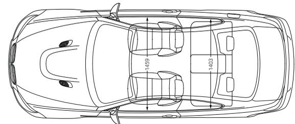
All dimensions of the technical drawings in millimetres. Luggage compartment capacity (VDA method): 430 litres.
