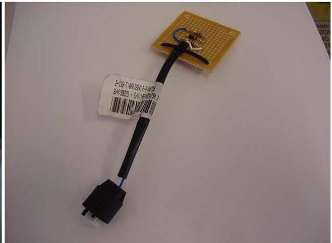
I didn't really see the point in installing the actual mat under the removable cushions of the Recaro. It may have worked but I would have had to drill a hole in the seat shell for the connector to reach under the seat and the mat isn't that rugged anyway. So, I made a circuit that fools the electronics. It's really very simple. See the closeup in the next picture and the schematic. The hard part was getting a
