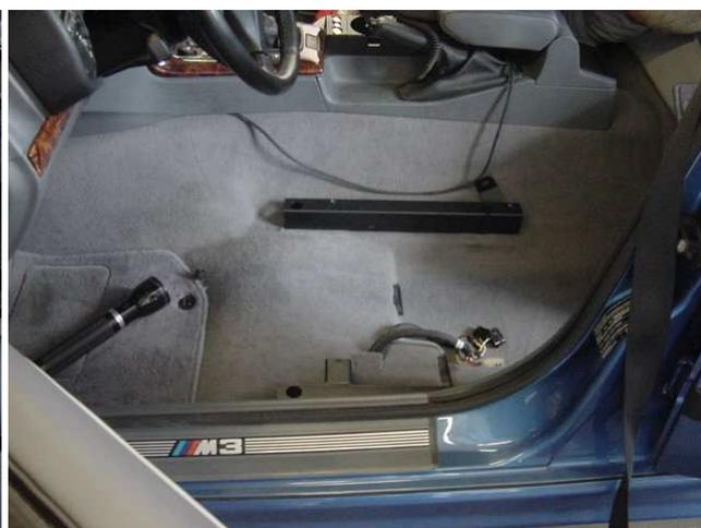
The drivers side will get sliders too but this gives an idea of the mounts used. The slider goes on top of this solid mount and adds 1 inch in height. Note the tab to mount the new inner lap belt and the factory receiver and tensioner.
