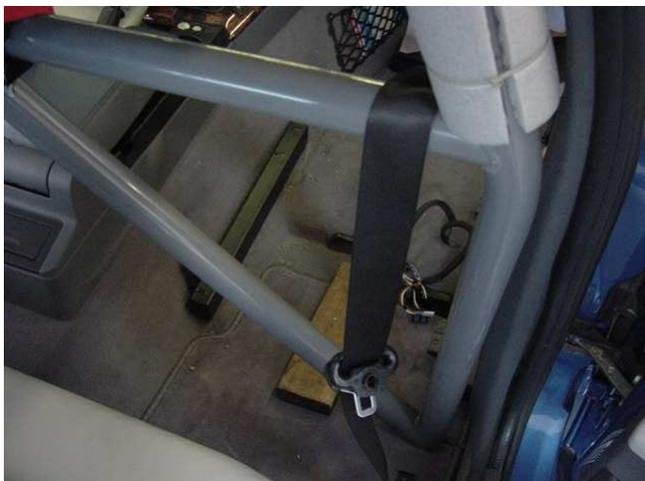
Here the seats are removed and the drilling for mounting the anti-submarine straps is getting done. Mounts are test fit for drilling to attach the Recaro brackets.
