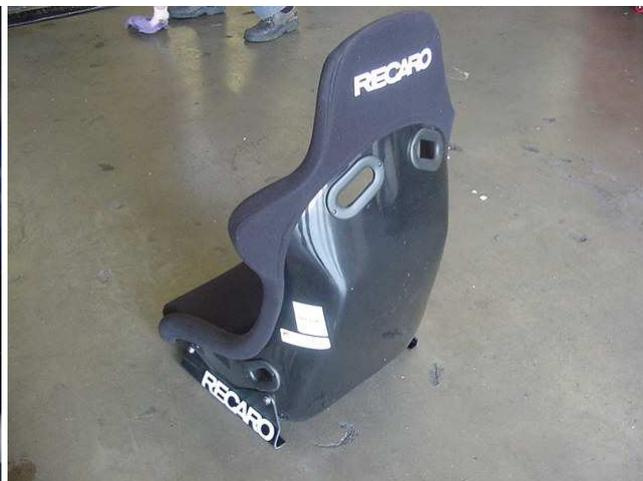
This is the back of one of the Recaro Pole Positions. The stock power electric sport seats with power lumbar and heating elements weighed 67 pounds. Together the Recaros cut a touch over 100 lbs off the car.
