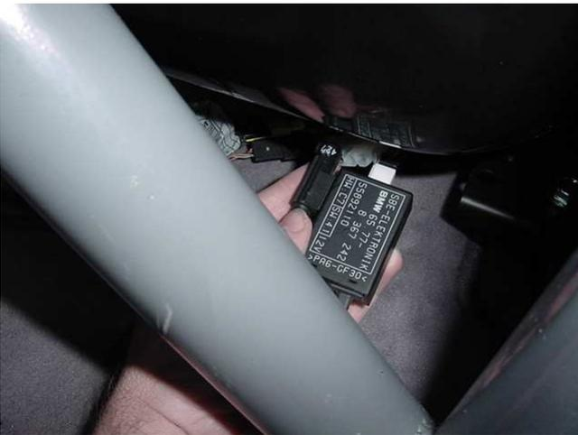
The stock seats incorporate a resistive mat that lets the SRS computer know if there is a passenger. Then the airbag will inflate or not on the passenger side in the event of an accident. Either move the sensor control module from your stock seats to the racing seat and the mat isn't that rugged anyway. So, I made a circuit that fools the electronics. It's really very simple. See the closeup in the next picture and the schematic. The hard part was getting a
