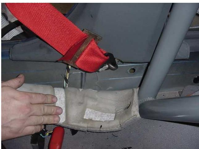
The new TRW Sabelt 6 point harness lapbelt mounts to the same bolt as the retracting seatbelt mechanism on the outboard side. Minor trimming of the B-pillar cover needs to be done to remove the factory bolt and put the eye bolt in to hold the stock mechanism and the new Sabelt piece.
