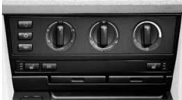
The E39 IHKR is a single zone system that regulates the temperature of the cabin based on the occupants desired temperature, selected by a temperature setting dial. Blower control, air distribution settings and stratification flap are manual.
