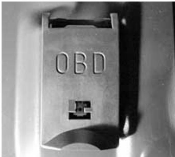
The cap to the OBD II connector contains a bridge that links KL 30 to TXD and TXD II. This is to protect the diagnostic circuit integrity and prevent erroneous faults.
