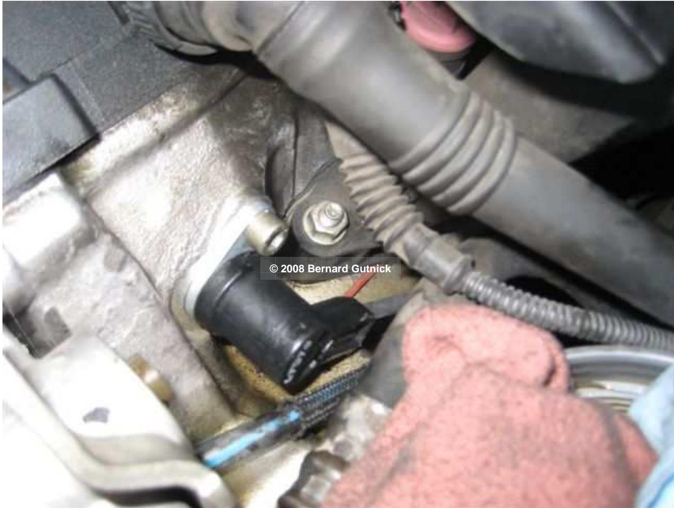
Loosen screw with allen wrench
