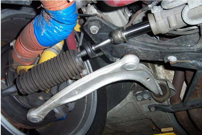
4. Undo the nut on the end of the steering rack shaft until it is completely disconnected. Do not change the position of the toe adjusting nut.
