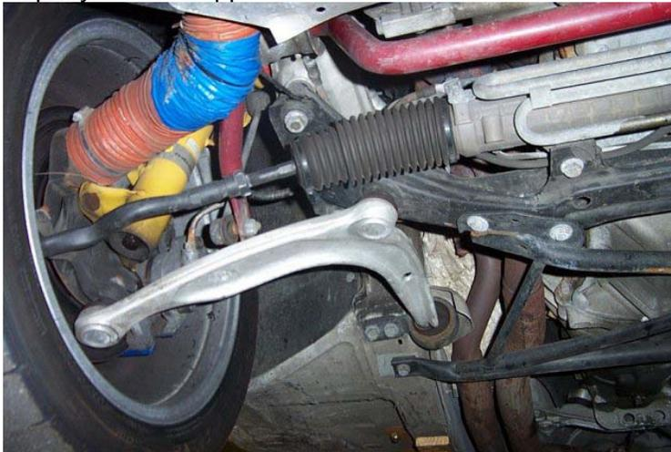
2. Remove/cut off the metal retaining bands. They will not be re-used.
