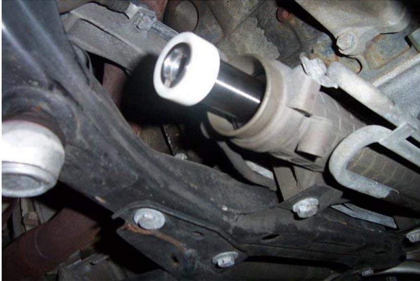
6. Put on the new locking plates (supplied in kit). Align locating tab with the groove in the rack. Reattach the tie rod end.
